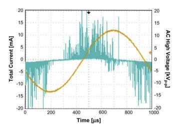
**Fig. 7.** Waveform of AC high voltage and total current for generation of the uniform slide discharge (negative DC high voltage  $-10\,\text{kV}$ , AC high voltage  $25\,\text{kV}_{\text{p-p}}$ ,  $2.0\,\text{mm}$  inner diameter,  $20\,\text{mm}$  capillary).
