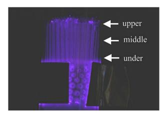
**Fig. 12.** Photographs of honeycomb discharge (AC 25 kV $_{p-p}$  1 kHz, DC -15 kV 2 mA,  $N_2$  gas 3 L/min, 2.0 mm inner diameter, 20 mm capillary, camera exposure time 4 s).
