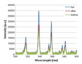
**Fig. 15.** Wavelength vs. emission intensity (AC 30  $kV_{p-p}$  1 kHz, pulse -10 kV, 1 kHz, air 3 L/min. 2.0 mm inner diameter. 20 mm capillary).
