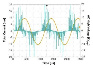
**Fig. 6.** Waveform of AC high voltage and total current for generation of the uniform slide discharge (negative DC high voltage -12.5 kV, AC high voltage 20 kV<sub>p-p</sub>, 2.0 mm inner diameter, 20 mm capillary).
