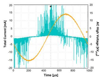
**Fig. 8.** Waveform of AC high voltage and total current for generation of the uniform slide discharge (negative DC high voltage -8 kV, AC high voltage 30 kV<sub>p-p</sub>, 2.0 mm inner diameter, 20 mm capillary).
