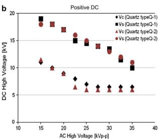
**Fig. 4.** Relationship between DC and AC high voltage for generation of the uniform discharge plasma. Capillary length, 20 mm; Q-1, 1.0 mm; Q-2, 2.0 mm inner diameter; Vc, the starting voltage; Vs, the maximum voltage (the flashover voltage).
