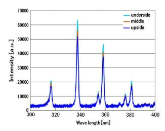
Fig. 13. Wavelength vs. intensity (AC 25  $kV_{p-p}$  1 kHz, DC -15 kV 2 mA,  $N_2$  gas 3 L/min, 2.0 mm inner diameter, 20 mm capillary).
