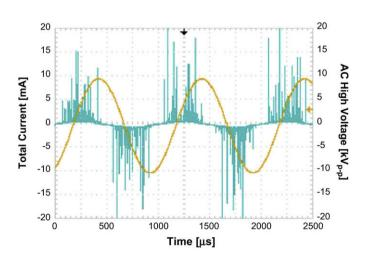
**Fig. 5.** Waveform of AC high voltage and total current for generation only packed bed discharge (negative DC high voltage 0 kV, 2.0~mm inner diameter, AC high voltage  $20~\text{kV}_{\text{p-p}}$ , 20~mm capillary).
